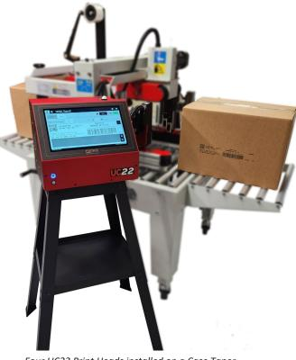
Four UC22 Print Heads installed on a Case Taper
