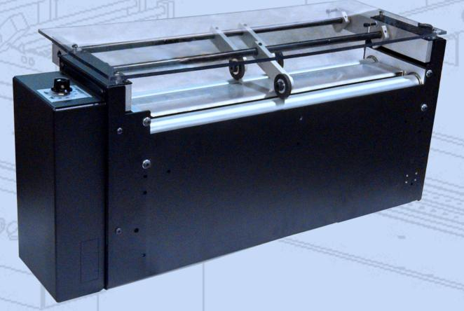
Walco Systems divert gates offer a reliable solution for your product verification needs. A lightning fast air-actuated door provides defective or incorrect pieces a route to be removed from the product stream. Spring loaded rollers allow more rigid pieces to be reliably diverted. Oversize frames and bearings provide reliable operation, and non proprietary replacement parts ease the cost of service.
