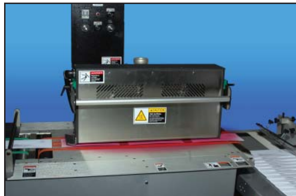
Specially designed bulbs reduce glare and direct most infrared energy towards the ink pattern. This means lower power settings can be used, reducing energy consumption and extending bulb life.
