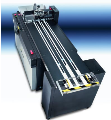
Model 7000 ink jet base with heat-resistant option
