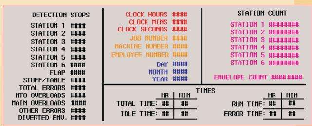
Information on the current job that is running on the inserter can be brought up on the inserters screen (Operator Interface). The inserter will keep track of the error stoppages, operator stoppages, and station pull quantity. Run time, error time, and idle time will also be kept.
