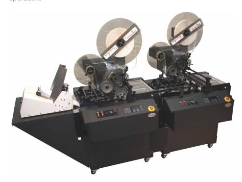
The CME- Ameritek Tabber can also be configured as a Dual Headed Tabber. This system can tab on the leading (toe) and trailing (heel) edges of a booklet in a single pass. The Dual Headed Tabber can run in-line or off-line as a system, or the Tabbers can be unlocked and used as stand-alone units.
